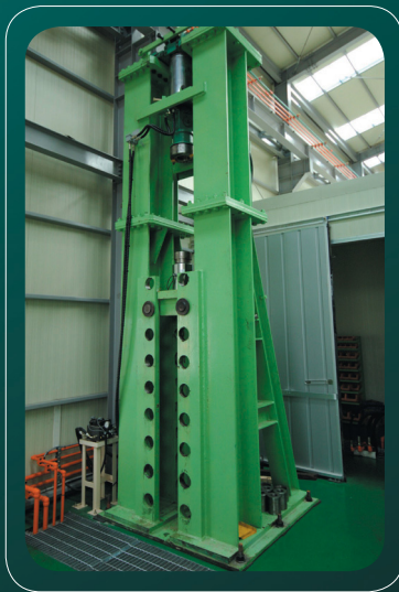
Static calibration test stand for correct measurement
